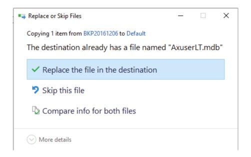
Select **Replace the file in the destination** to overwrite the empty database with the populated database from the backup. Once this has completed, go to the Axiom Lite installation disc and open the **Upgrade** folder. Re-run the latest Service Pack found in the Upgrade folder. This will sync the old database to the new software version. In the example shown below the service pack is;
