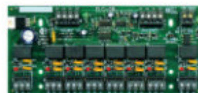
The URC-ELV8-B relay output module is designed for mounting in the standard ENCL1 enclosure. Available individually or as part of the URC-2008.
